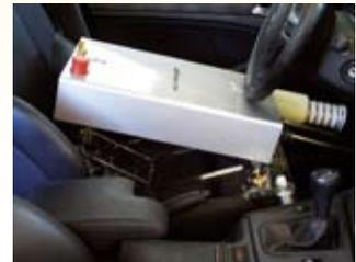
Actuator for EMC measurement
